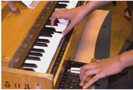
Figure 1: Playing the Ondes Martenot using the keyboard: right hand controls the pitch of the note while left hand adjusts the volume by pressing the intensity key.
